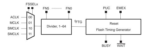
The flash timing generator can be sourced from ACLK, SMCLK, or MCLK. The selected clock source should be divided using the FNx bits to meet the frequency requirements for f<sub>FTG</sub>. If the f<sub>FTG</sub> frequency deviates from the specification during the write or erase operation, the result of the write or erase may be unpredictable, or the flash memory may be stressed above the limits of reliable operation.
